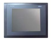
The microprocessor touch screen control can be programmed to display in four languages. It has features for programming any wash activity to meet today and tomorrow's demand for water treatment of textile fiber and garments. It is the most flexible control system yet developed for the stand-alone commercial and industrial washers in the industry and has a proven track record for reliability.
